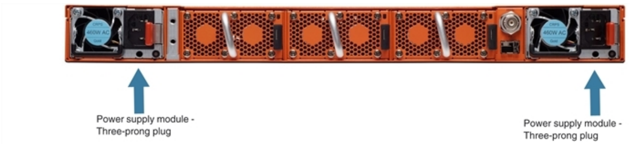
Figure 2 Connecting AC Power (GigaVUE-HCI)
